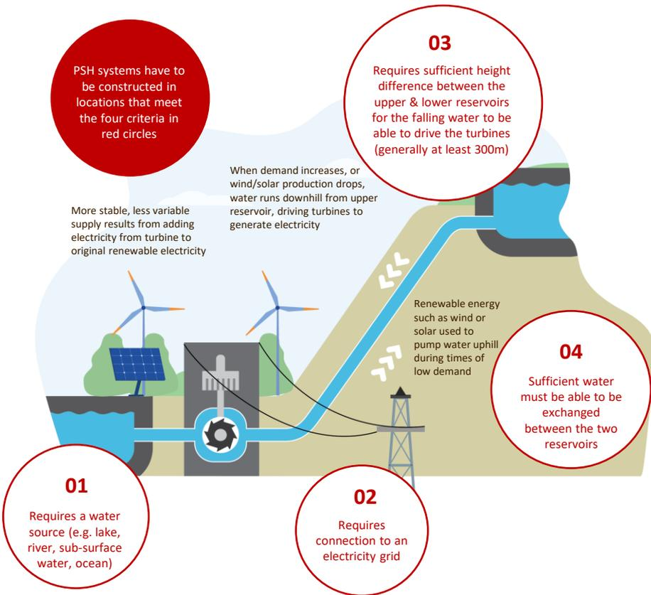
Figure 2 Schematic of a typical PSH configuration (Source: Adapted from ARENA (2021))
